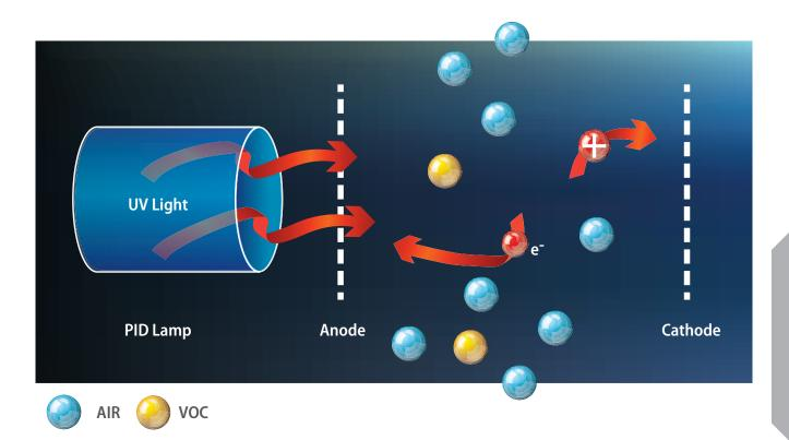
Most substances can be ionized, some more easily than others. The ability of a substance to be ionized is measured as ionization potential (IP) using an electron volt (ev) energy scale. This scale generally runs from a value of 7 to a value of approximately 16. Substances with an ev rating of 7 are very easy to ionize; substances with an ev rating of between 12 and 16 are extremely difficult to ionize. IP ratings of some common substances include:
